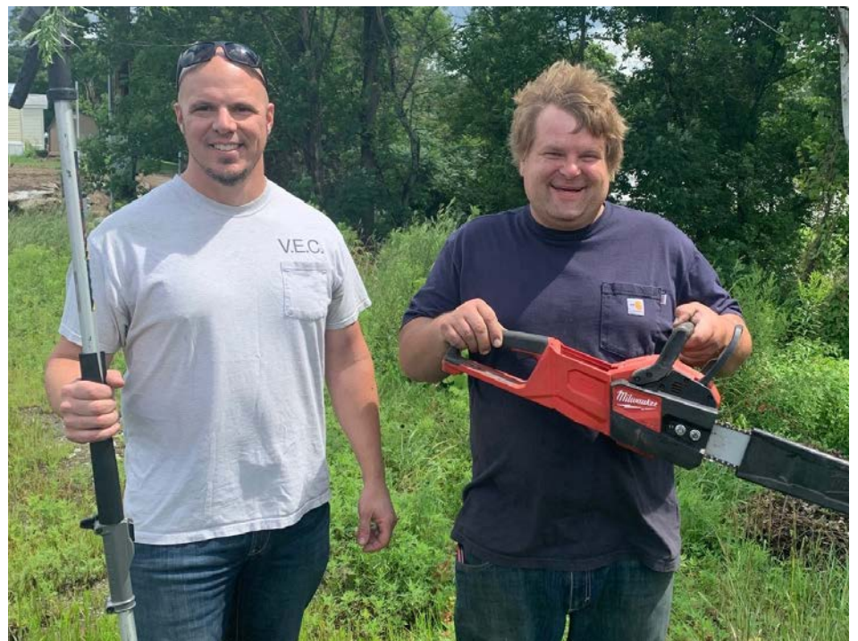
VEC Safety Technician David Young, left, holds an electric sickle bar brush cutter. At right is Substation Technician Dan Hinton with an electric chainsaw. When VEC crews operate this type of equipment they wear full personal protective equipment and we encourage our members to do the same.
