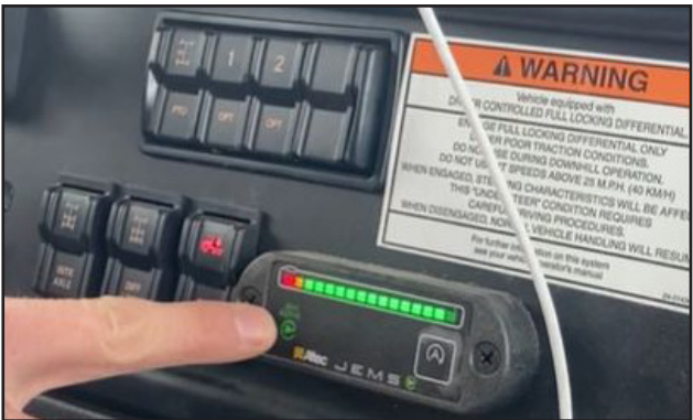
VEC's new hybrid bucket trucks, above, look like traditional trucks, but electricity powers the boom. Below, the truck's large battery system, and its interaction with the truck's diesel engine, can be controlled on this simple dashboard display.
