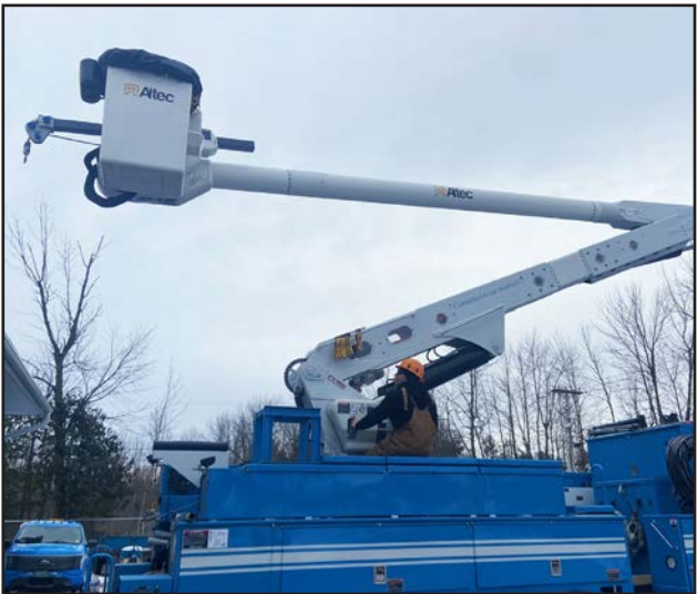
VEC's new hybrid bucket trucks, above, look like traditional trucks, but electricity powers the boom. Below, the truck's large battery system, and its interaction with the truck's diesel engine, can be controlled on this simple dashboard display.
