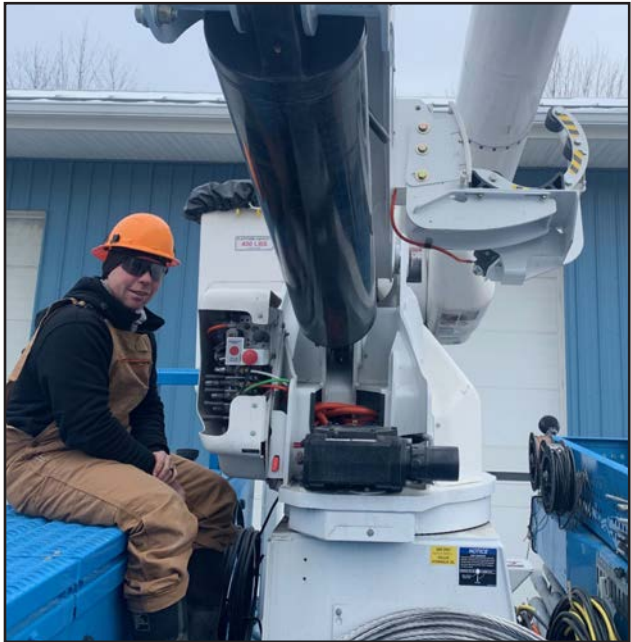
Grand Isle District lineworker Chris Connelley in the back of one of VEC's new hybrid bucket trucks. The trucks make less noise when they are on site working, and fuel use is reduced significantly.
