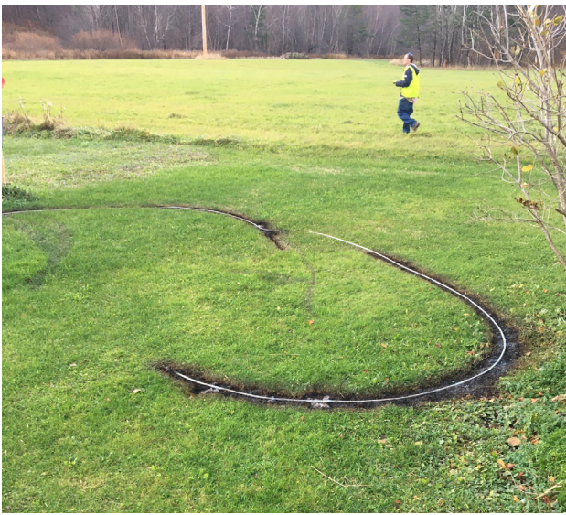
Above: This line that came down on North Hill Road in Westfield was energized when it landed on the ground, burning the grass. Such lines may not make any noise even when they remain energized. Walking near fallen lines, if they are live, can cause injury and even death if the electricity travels up a person's leg, through their body, and back down the other leg.
